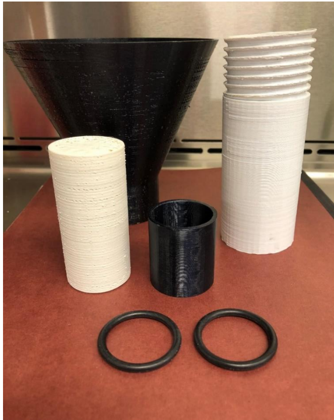
Figure 3: The pieces of the funnel system, including the siphon funnel, holder for the filter, spacer, and rubber o-rings, along with one of the filters.
