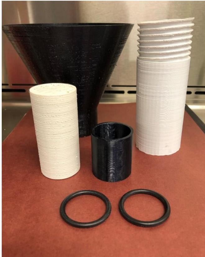
To test the volume of solution needed to activate the siphon of the funnel, 150 milliliters of water was added to the funnel, then water was added in 5 mL increments until the water began to flow through the funnel. To determine the volume of solution lost to the system, 500 milliliters of water were flowed through the funnel into a beaker and the volume in the beaker was recorded and subtracted from the initial 500 milliliters. Both processes were repeated three times.
