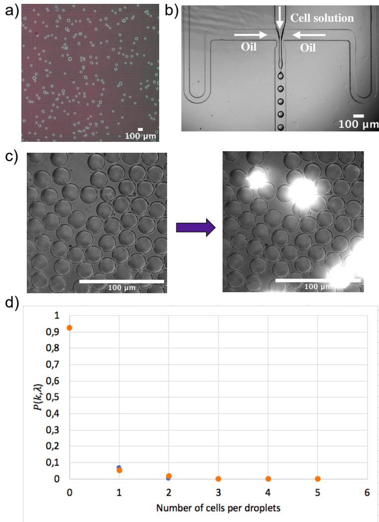
**Figure 2:** Microscopic images of the experiment and resultant graph. (a) Microscopic image of fluorescent cells in the hemocytometer ready for counting. (b) Microscopic image of the droplet generation in the microfluidic device. (c) Image of the microdroplets before and after fluorescence. (d) A plot of the probability of getting  $k$  number of cells per droplet based on  $\lambda$ .
