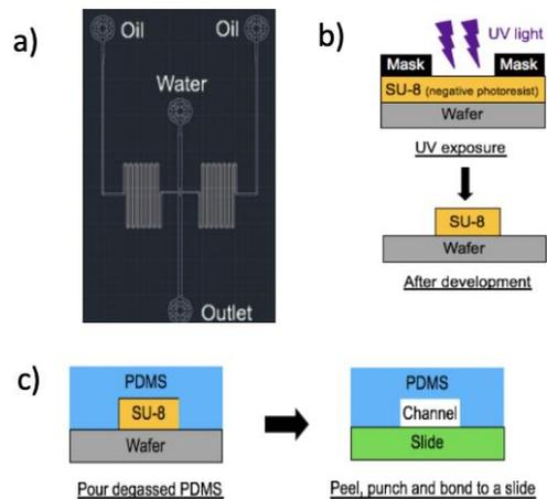
**Figure 1.** Schematics and images of the microfluidic device and fabrication. (a) Image of the device used for microdroplet generation. (b) Schematic showing the UV exposure and development of SU-8. (c) Schematic showing the steps of soft lithography.
