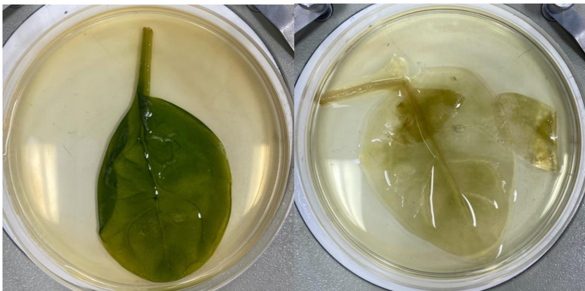
Figure 3.2: The left leaf was statically soaked in DI water for one week while the right leaf was statically soaked in 10% SDS for one week. The SDS has dissolved much of the cellular content, resulting in the leaf's translucency compared to its still-green DI control.
