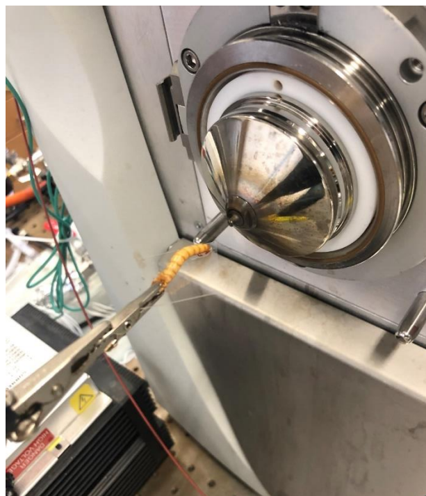
Figure 3: “Bug-Spray” extraction technique, in which the insect is mounted on the clip electrode on a glass coverslip instead of a paper triangle.
