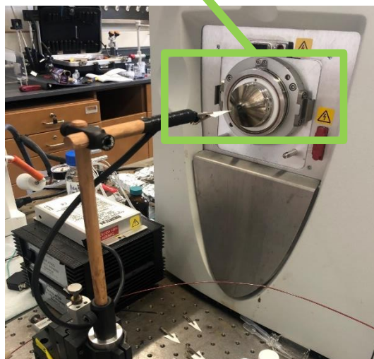
Figure 4: Example of PSI-MS schematic. A ThermoFisher LTQ XL Linear Ion Trap Mass Spectrometer was used.
