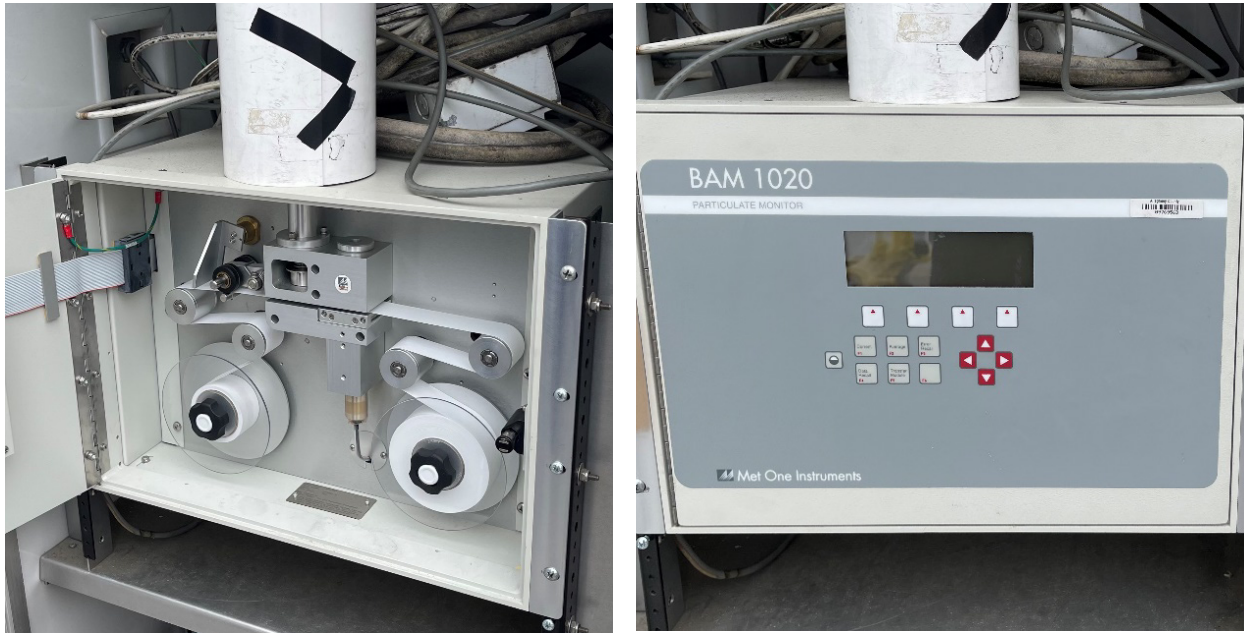
Figure 4. The Met One BAM 1020 particulate monitor. This instrument is currently inactive but remains on the roof of the Lawrenceville monitoring site.
