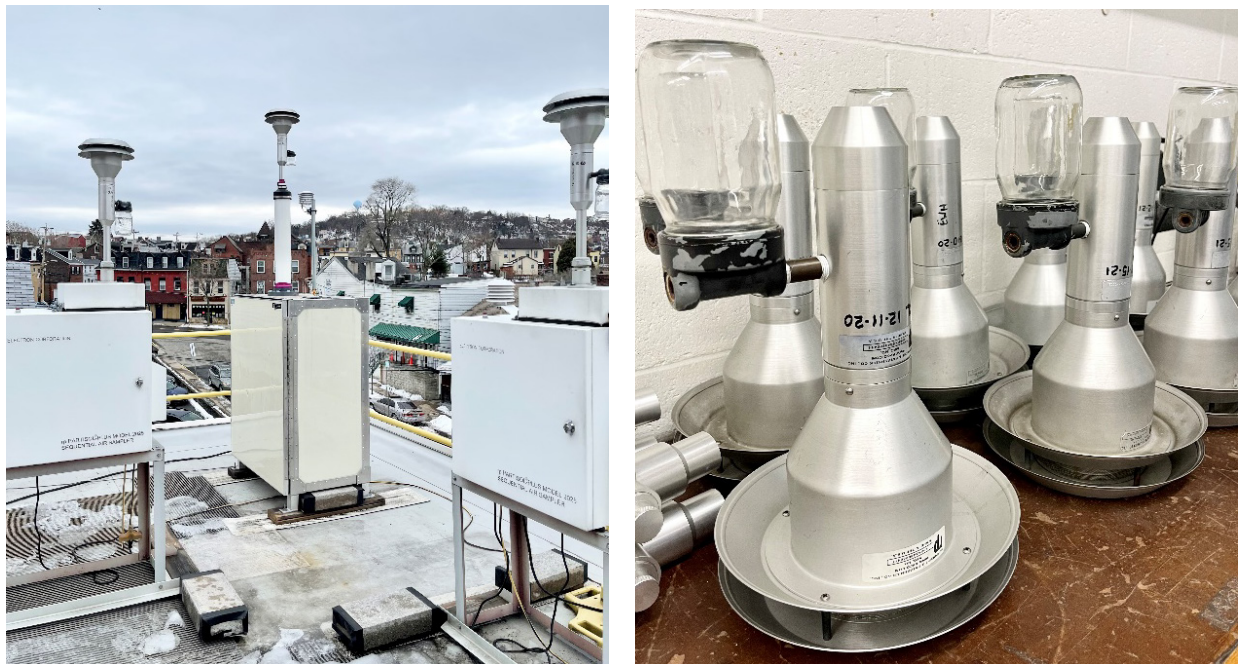
Figure 5. Several of the particulate matter air monitors in use at the Lawrenceville monitoring site (left) as well as the inlets that are used to bring ambient air into the monitoring device (right).
