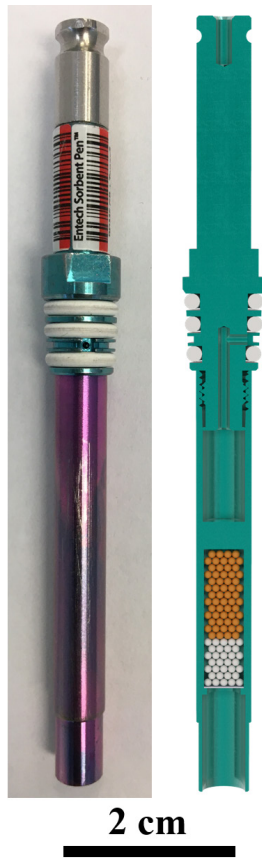
Figure 5.4 Photograph and render of an FSP showing the internal sorbent beds.
