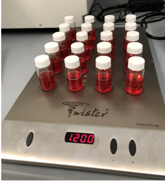
Figure 3.1. Sample vials containing human whole blood sample stirring on a magnetic stirring plate.
