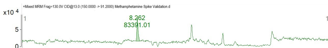
Figure 5.8 Extracted MRM chromatogram of the quantifier ion for methamphetamine spiked into synthetic urine at the cutoff concentration of 500 ng/mL.
