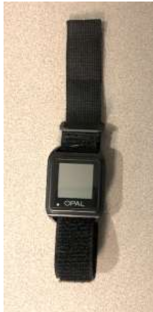
Figure 3. Wearable inertial measurement unit (Opal wearable sensors, APDM Inc., Portland, Oregon).
