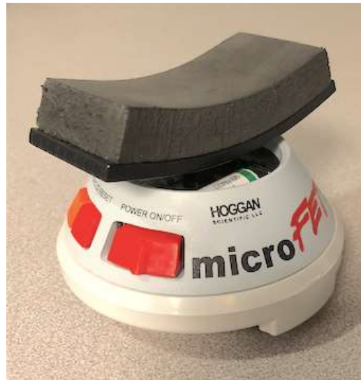
Figure 5. The Hoggan Scientific MicroFET 2 handheld dynamometer (Hoggan Scientific, Salt Lake City, UT) was used to measure maximum force output of the hip lateral rotators, extensors, and abductors.
