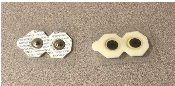
Figure 2. Electrodes were disposable, self-adhesive HEX dual snap, pre-gelled, silver chloride electrodes with 2.0cm of fixed inter-electrode distance (Noraxon USA Inc., Scottsdale, AZ).
