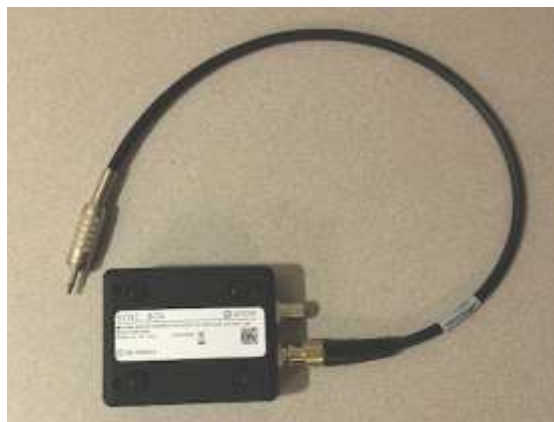
Figure 4. A sync box (APDM Inc., Portland Oregon) was used to synchronize sEMG and kinematic data to determine muscle activity during the SLST.
